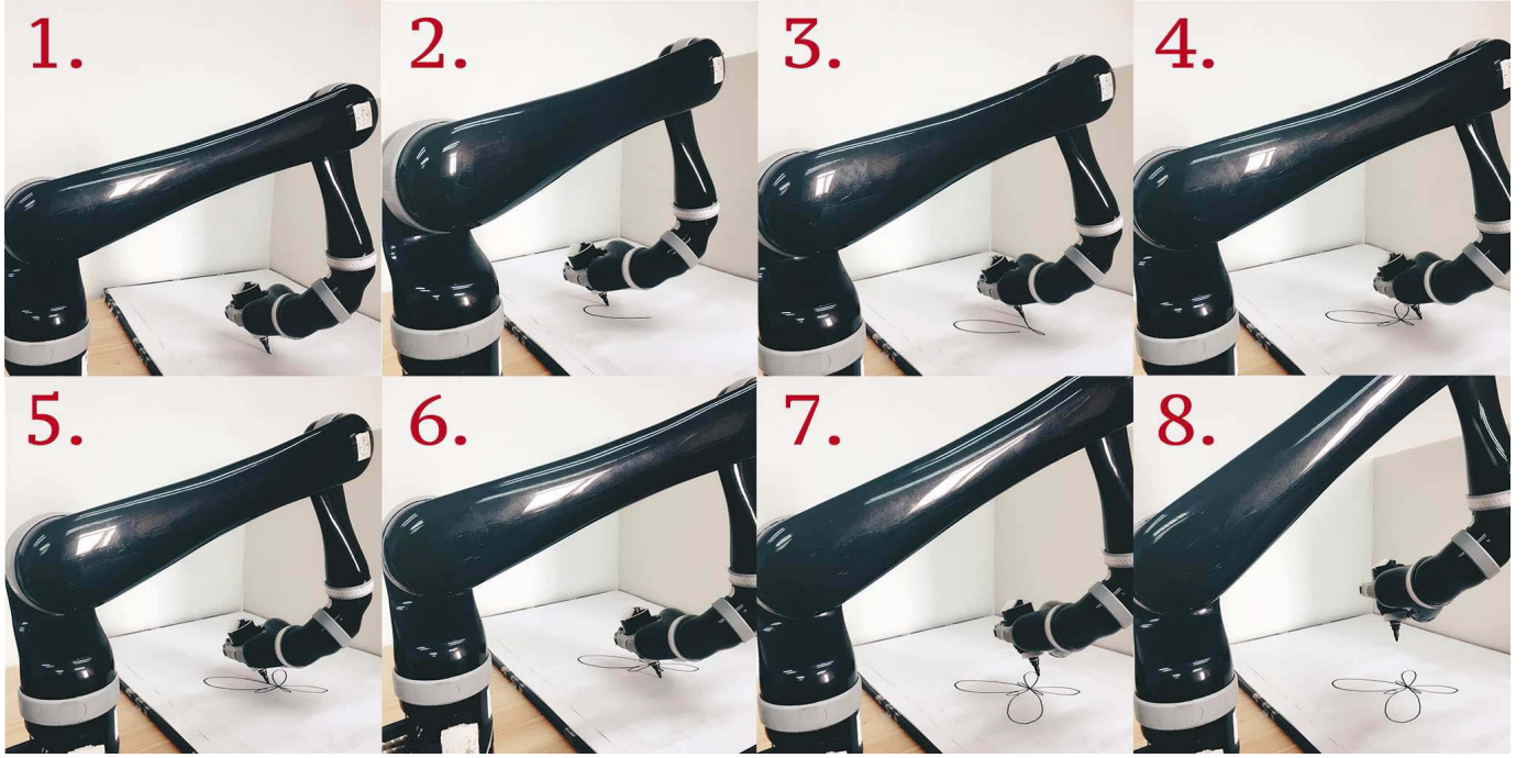
Fig. 9. Experimental process of a Kinova JACO 2 manipulator for tracking a butterfly path controlled by VPNN.
